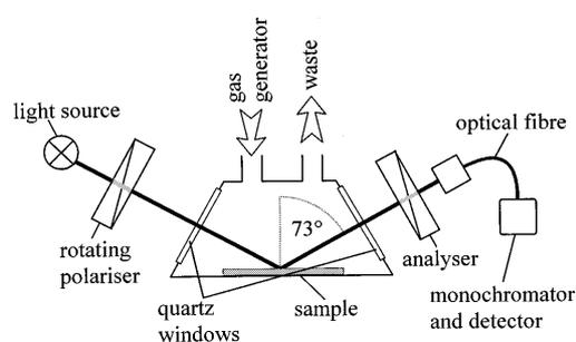
**Fig. 1** Schematic set-up for the ellipsometrical in-situ characterization of the changes in thickness and refractive index of thin polymer films in contact with organic vapours
