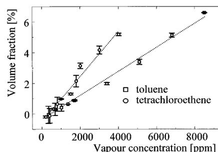
**Fig. 5** Volume fraction of toluene and tetrachloroethene in the polymer film, depending on the vapour concentration
