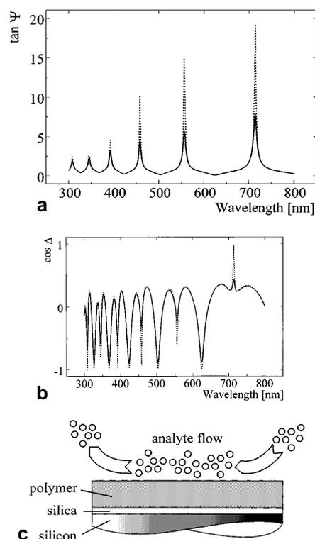
**Fig. 2a, b** Ellipsometric angles versus wavelength for a PDMS film on a thermally oxidized silicon wafer in contact with dry air: **a**  $\tan \Psi$ ; **b**  $\cos \Delta$ . The *solid lines* indicate the measured data. The *dotted lines* represent the data obtained from the layer model in **c**. Details are given in the text
