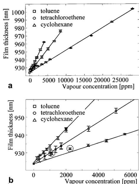
**Fig. 3** **a** Change of the thickness of a PDMS film versus analyte concentration. **b** Zoomed portion of **a** for the concentration range up to 6000 ppm
