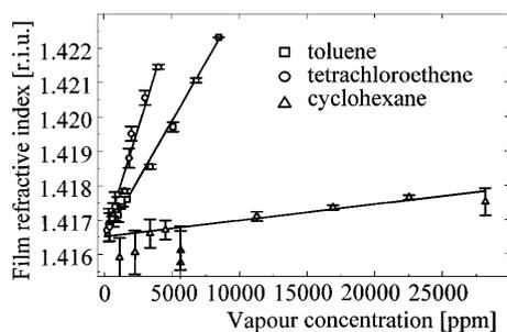
**Fig. 4** Refractive index of the resulting mixture phase *PDMS*/toluene, *PDMS*/tetrachloroethene, and *PDMS*/cyclohexane at 589.6 nm and 20°C versus analyte concentration
