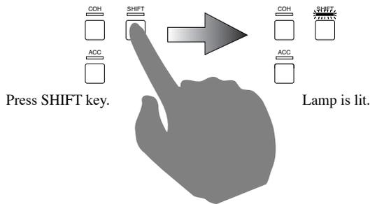
When the SHIFT LED is lit, press the rotary encoder change key.
