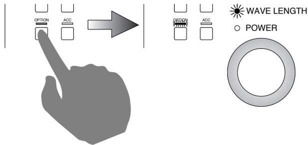
If the LED is not lit, change the rotary encoder change key (toggle action) to the wavelength side.
