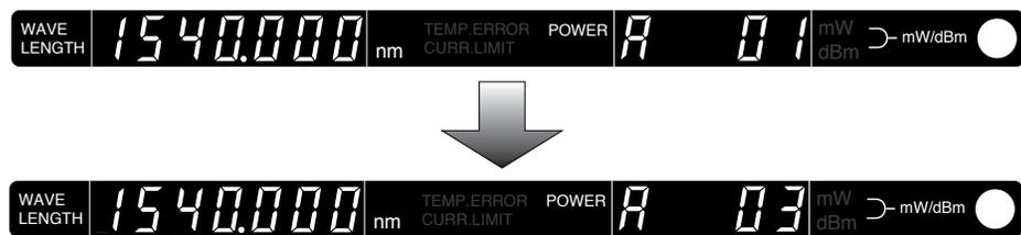
GP-IB address and delimiter is saved to memory after setting. SHIT LED goes off and display shows output power.
