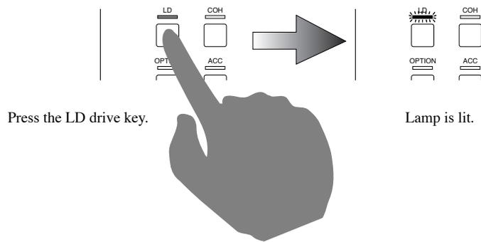
When the key is pressed, the LD drive LED is lit and current is supplied up to the set current by APC mode. The set optical output power at power start up is -40.00dBm/0.00mW.
