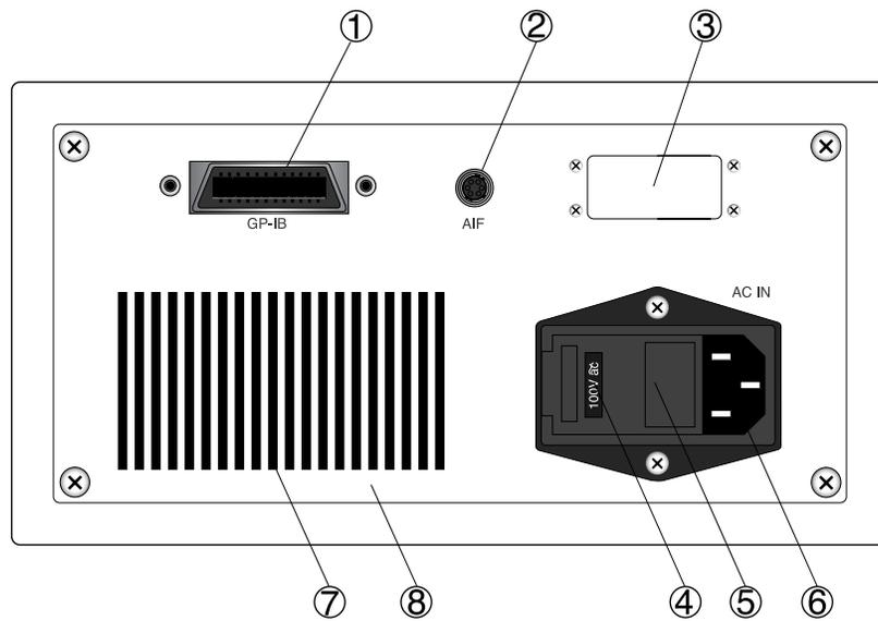
**(1) GP-IB connector (Refer to 10-5 GP-IB)**
