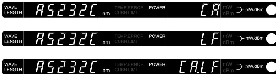
RS-232C delimiter can be changed by turning on power while holding OPTION or APC key. The delimiter setting is kept effective even though unit is OFF.
