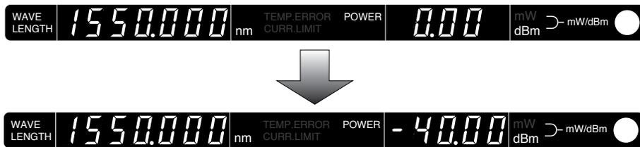
The protection circuit prevents an instantaneous loss of current in the LD; therefore, it will take a moment after pressing the LD drive key for the LD to go out. Injection current is not completely shut off until the LD indicator goes out—please pay special attention to the indicator and wait until it is out before shutting off the power source.
