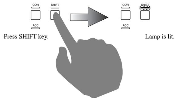
When the SHIFT LED is lit, press the wavelength calibration key.
