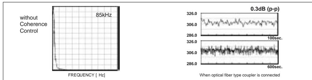
TSL-210 has the spectrum linewidth 2-step control so as to configure a stable measurement system even in such a case.
