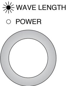
When the LED is not lit, turn the rotary encoder change key to the wavelength side.
