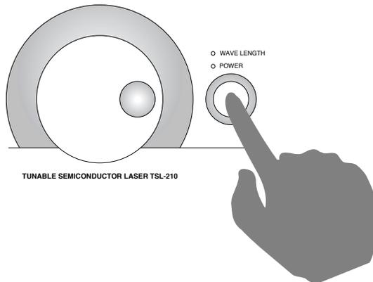
After making sure the wavelength setting LED is lit, set the wavelength by the rotary encoder. The wavelength reading exactly follows the rotations of the encoder dial when the dial is gradually turned, while the reading changes in unit of nm when the dial is turned fast. When the wavelength display stops changing, it means that the wavelength is set in a range of 0 and 1nm. The setting will complete in 170 msec.
