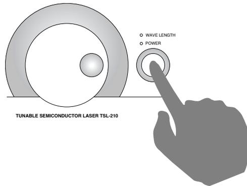
If the key is pressed, minimum step digit which is currently set on the wavelength display panel is flickering. Select minimum step digit by rotating rotary encoder. (Setting range is 10nm – 1/1000nm)
