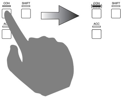
When the key is pressed, the coherence control LED is lit, to show that the coherence control is ON. To turn OFF the coherence control, press the coherence control key once again.
