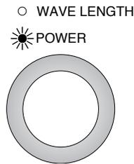
If the LED is not lit, toggle the rotary encoder change key (toggle action) to the optical output power side.
