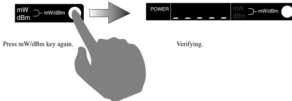
Upon completion of writing, the symbol "\_" is replaced with the optical output power value and shift lamp goes OFF.
